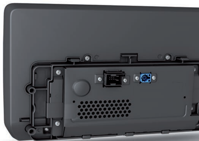
Display unit for front information display and operating unit control unit J685
